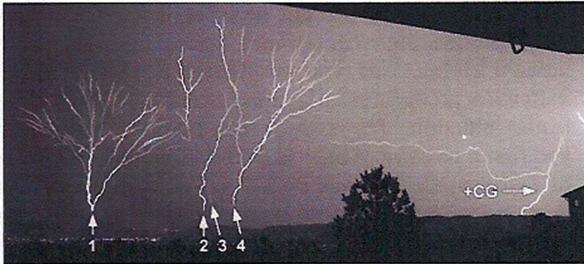
Figure 4. High-definition video image (60 ips) showing the preceding +CG return stroke channel and self-propagating upward leaders developed from all four towers.
