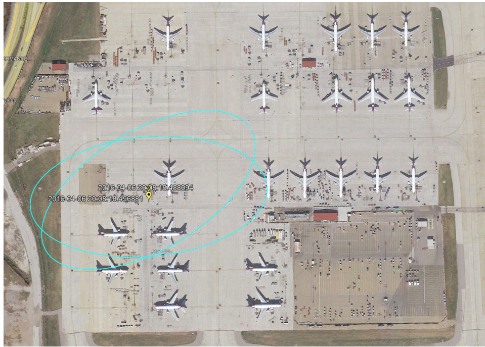
Fig. 7. Reported NLDN lightning strike locations for two strokes on April 6, 2016 within an airplane staging area at the Memphis FedEx World Hub. Two FedEx employees experienced lightning-related injuries associated with these events, which occurred within an area covered by a DAS array. DAS devices are located on utility poles immediately adjacent to the nose of each pictured airplane.
